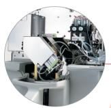
**Close structure** Shield from interference: EMI, dust, etc.
