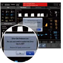
To ensure the patient is ventilated at all times the WATO EX-65 has a unique driven gas auto-switch function. Should the primary ventilator driven gas be lost the device will automatically switch to Air (or  $O_2$ ; dependent on device configuration) without interruption to mechanical ventilation.
