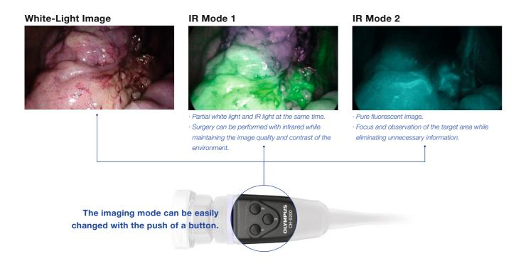
The VISERA ELITE II is a next-generation system that uses components other than the light source and the telescope in common with the normal observation system. IR observation is possible just by adding a dedicated light source and telescopes. The new dedicated IR telescope provides an image optimized for IR transmission with an ED lens.
